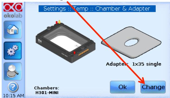
Select the chamber you have by pressing on the arrows '<' and '>' on the edges of the screen until you find the chamber you have. Once you find your chamber press 'NEXT' to access the inserts and follow the same procedure until you find the insert you have. Press 'OK' to select it. See an example here:
